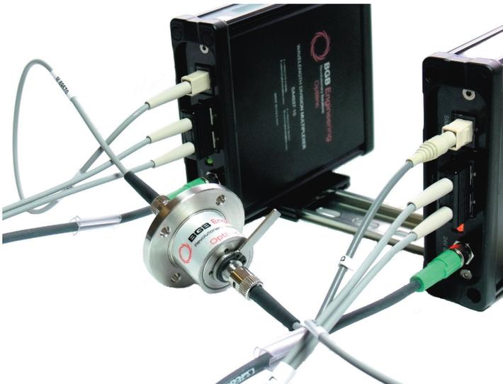
The new BGB WDM (Wave Division Multiplexer) is designed to complement and enhance BGB's Optilinc FORJ to convert two fibre (duplex) systems to a single fibre multiwave length system (simplex).
